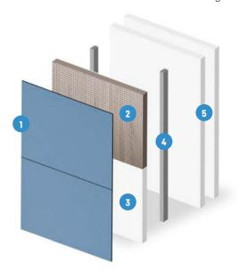
The multi-part wall construction with integrated, acoustically beneficial material as well as the glass door with high-quality floor lowering seal and optional magnetic closure also contribute to the ideal sound insulation of the se:cube.
